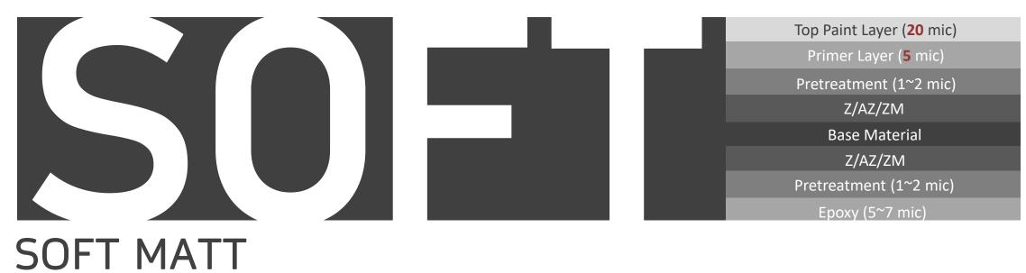
SOFT is a Polyester based coating with soft surface texture which is created by special paint hardening and wrinkle construction. SOFT has a micro grain that secures shimmering appearance of silk touch.
